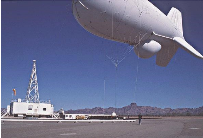
Figure 8 Air force tethered aerostat radar
