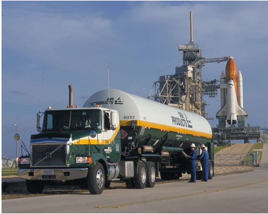
FIGURE 1. Helium is used for purging liquid hydrogen systems in space launch vehicles.
